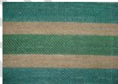
Fig. 4 (a) Diamond twill mat (Kenaf rope) Source: Osei and Osei-Poku(2014)
