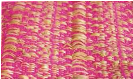
Fig. 3 (a) Twill weave mat (sisal fibre) Source: Osei and Osei-Poku(2014)
